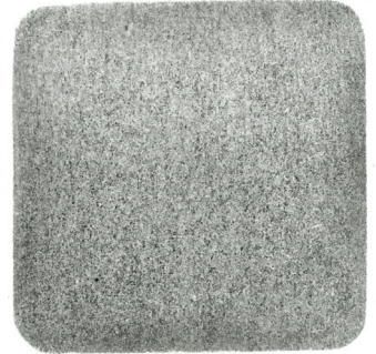
FIGURE 3 – KILLED STEEL (C 15 E)
